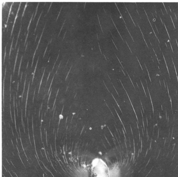
Figure 3 Distributed crazing near a crack tip in PMMA at 105 °C.
